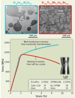
Improvements in mechanical properties (e.g., tension ductility) have been confined almost exclusively to Zr-Ti-Be-based BMGMCs, which has limited the scope of applications.
