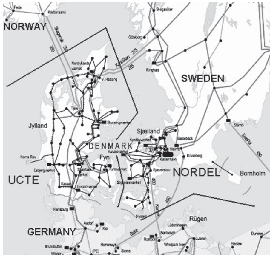
Figure 1. Transmission system of Denmark, presently divided into two synchronous areas
