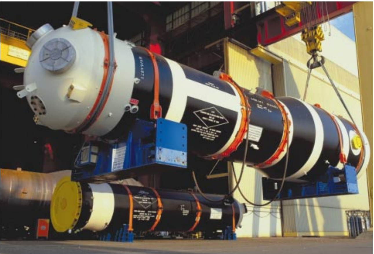
Steam generator & pressurizer
