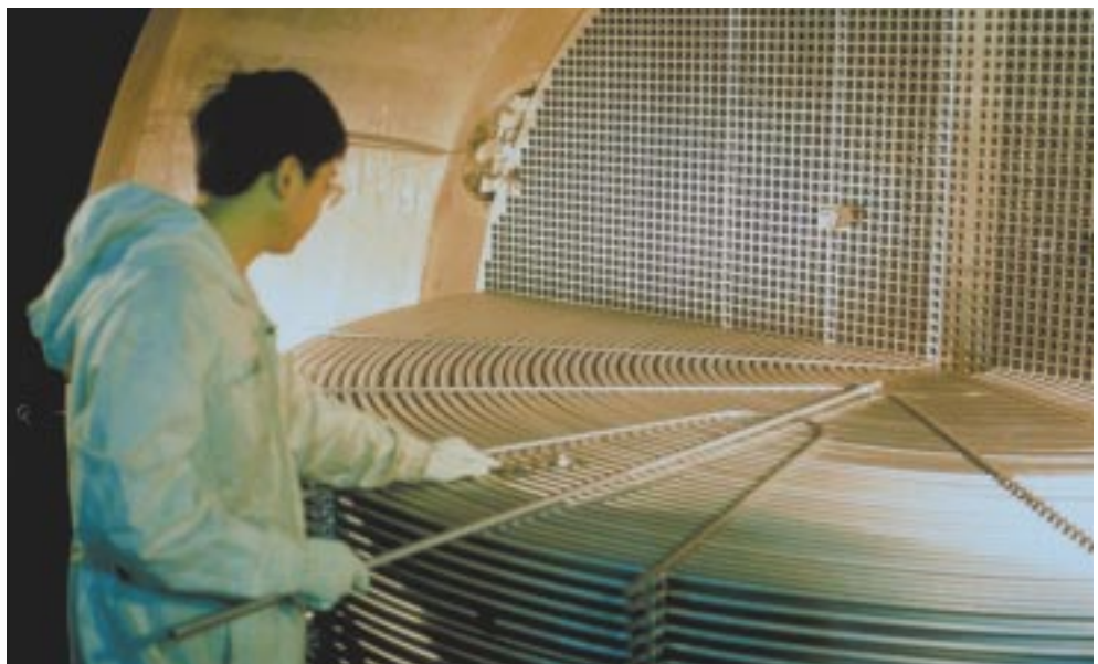
Steam generator tubing and installation of anti-vibration bars in China
