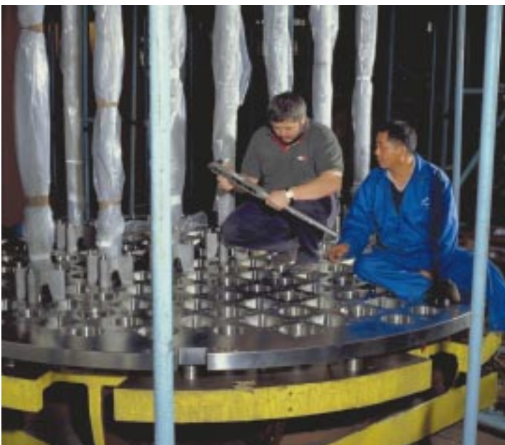
Lower internals core support plate
