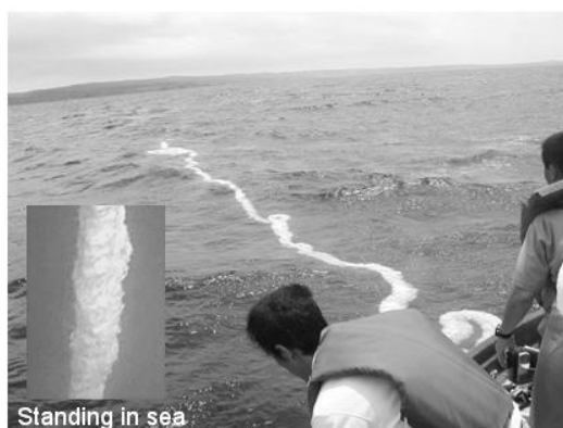
Figure 6 Recovery of braid adsorbent in marine experiment at Okinawa.
