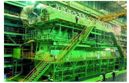
Figure A.15. The Wartsila-Sulzer RTA96-C 14-cylinder engine. 27 m long and 13.5 m high. http://www.wartsila.com/
