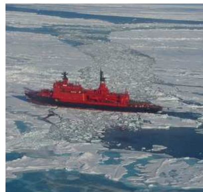
Figure 20.30. The nuclear ice-breaker Yamal, carrying 100 tourists to the North Pole in 2001. She has two 171 MW reactors, and her motors can deliver 55 MW. Photo by Wofratz.
