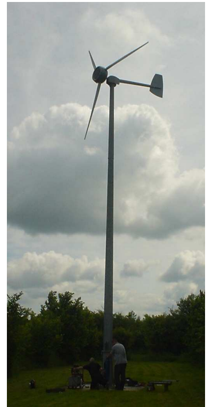
Figure B.11. A 5.5-m diameter Iskra 5 kW turbine [www.iskrawind.com] having its annual check-up. This turbine, located in Hertfordshire (not the windiest of locations in Britain), mounted at a height of 12 m, has an average output of 11 kWh per day. A windfarm of machines with this performance, one per 30 m × 30 m square, would have a power density of 0.5 W/m 2 .
