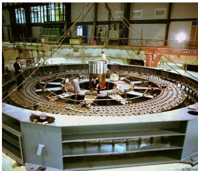
Figure 26.16. One of the two flywheels at the fusion research facility in Culham, under construction. It weighs 800 t. Spinning at 225 revolutions per minute, it can store 1000 kWh, and its energy density is about 1 Wh per kg. Photo: EFDA-JET. www.jet.efda.org .
