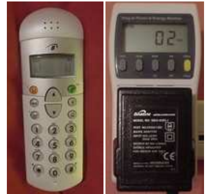
Figure 11.3. This lousy cordless phone and its charger use 2 W when left plugged in. That's 0.05 kWh/d . If electricity costs 10p per kWh then a 2 W trickle costs £2 per year.
