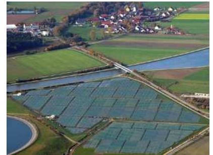
Figure 6.7. Solar photovoltaic farms: The 6.3 MW (peak) Solarpark in Mühlhausen, Bavaria. Its average power per unit land area is expected to be about 5 \text{ W/m}^2 . Photo by SunPower.
