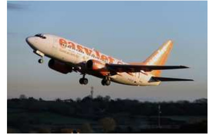
Figure C.11. Boeing 737-700: 30 kWh per 100 passenger-km . Photograph © Tom Collins.
