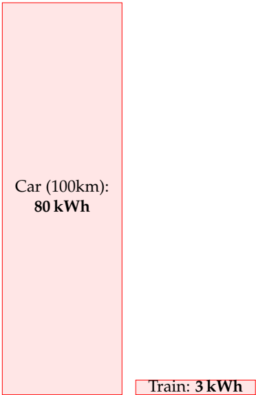
Figure 20.32. 100 km on a fully-occupied high-speed train, compared with 100 km in a single-person car.
