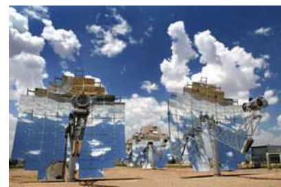
Figure 25.7. Stirling dish engine. These beautiful concentrators deliver a power density of 14 W/m 2 of land. Photo courtesy of Stirling Energy Systems. www.stirlingenergy.com
