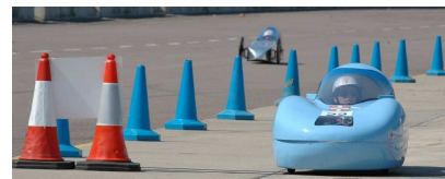
Figure 20.2. Team Crocodile's eco-car uses 1.3 kWh per 100 km . Photo kindly provided by Team Crocodile. http://www.teamcrocodile.com/
