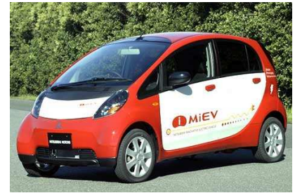
Figure 20.35. The i MiEV. From Mitsubishi Motors Corporation. It has a 47 kW motor, weighs 1080 kg, and has a top speed of 130 km/h.
