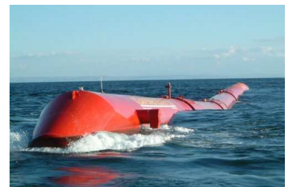
Figure 12.1. A Pelamis wave energy collector is a sea snake made of four sections. It faces nose-on towards the incoming waves. The waves make the snake flex, and these motions are resisted by hydraulic generators. The peak power from one snake is 750 kW; in the best Atlantic location one snake would deliver 300 kW on average. From Pelamis wave power www.pelamiswave.com .
