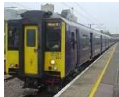
Figure 20.4. This 8-carriage stopping train from Cambridge to London, at its maximum speed of 100 mph (161 km/h), consumes 1.6 kWh per 100 passenger-km , if full.
