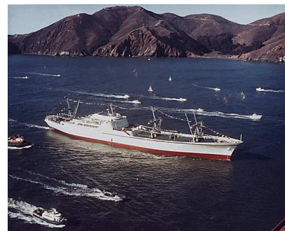
Figure 20.29. NS Savannah, the first commercial nuclear-powered cargo vessel, passing under the Golden Gate Bridge in 1962. She has one 74 MW reactor, and her motor can deliver 15 MW.
