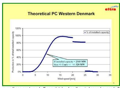
This power curve, by courtesy of ELTRA, illustrates the reality of operating the modern wind machinery on which UK hopes are founded.
