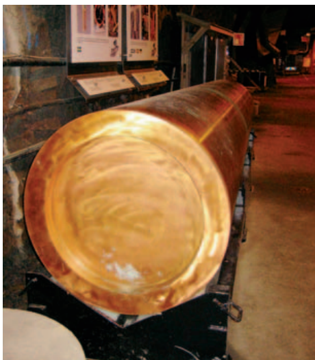
A copper-coated canister that weighs 25 tons and can contain two tons of spent nuclear fuel sits 450m below the ground at the site of a proposed nuclear waste repository in the southeastern Swedish town of Oskarshamn. – AFP
